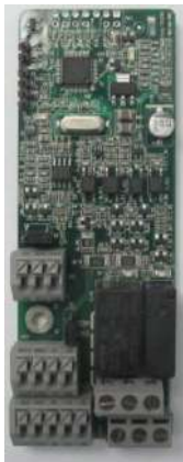
I/O expansion card 1 EC-IO501-00
