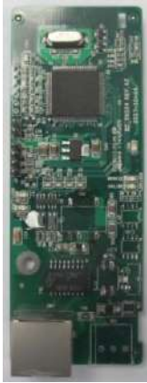
Ethernet communication card EC-TX504
