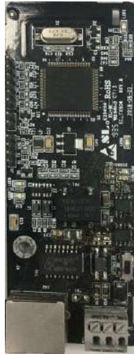
CAN-NET two-in-one communication card EC-TX511B
