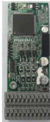
Multifunction incremental PG card EC-PG505-12
