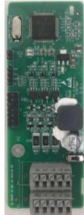
Simplified incremental PG card EC-PG507-12
