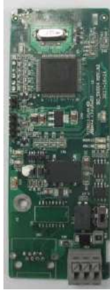
CANopen/CAN master/slave control communication card EC-TX505/511
