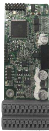
Resolver PG card EC-PG504-00
