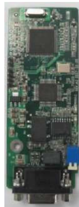
PROFIBUS-DP communication card EC-TX503
