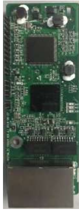
PROFINET communication card EC-TX509
