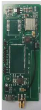
Bluetooth/WIFI communication card EC-TX501/502
