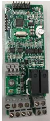
I/O expansion card 2 EC-IO502-00
