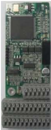
Incremental PG card with UVW EC-PG503-05
