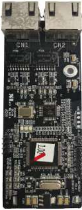
Ethernet/IP communication card EC-TX510/ EC-TX515
