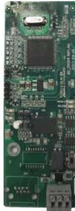
CANopen/CAN master/slave control communication card EC-TX505/511
