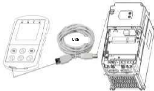
Figure 5-1 Connection of manual operator interface with EC100
